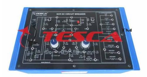
Power Electronic Training Board has been designed specifically to study the SCR as D.C. circuit breaker when the D.C. circuit exceeds specified limit. The set up works on 30V D.C. and permits the circuit breaker to be adjusted from 100mA to 1.8 Amp. This Training Board also includes Electronic Crow Bar circuitry to demonstrate the over voltage and over current trip under D.C. Condition.
