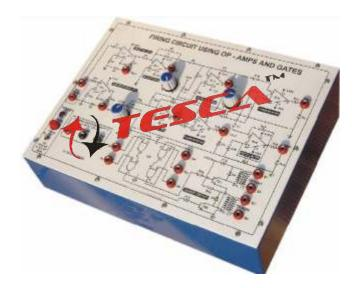
Power Electronic Training Board has been designed specifically for the study of the firing circuit for single-phase converter using Op-Amps and Gates.
