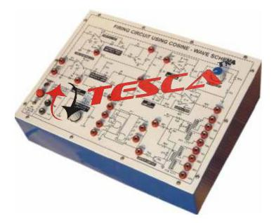
Power Electronic Training Board has been designed specifically for the study of the firing circuit for single-phase converter using cosinewave comparator scheme.
