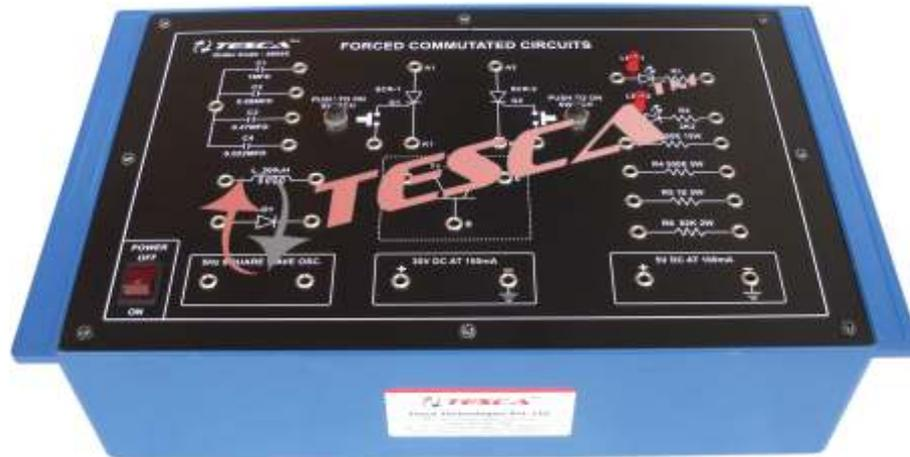
Power Electronic Training Board has been designed specifically for to study the forced commutated circuits.
