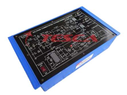
Power Electronic Training Board has been designed specifically for the study of the step down voltage commutated thyristorised chopper.
