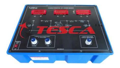
Specifically to study and Plot VI Characteristics of A Power MosFet. The board is absolutely self contained.
