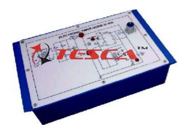
Power Electronic Training Board has been designed specifically for the study of Electronic Timer using IC-555. The board is absolutely self contained and requires no other apparatus.
