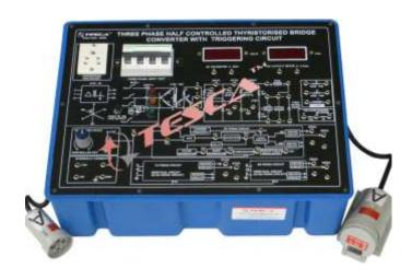
Power Electronic Training Board has been designed specifically for the study of Three Phase Half Controlled Thyristorized Bridge Converter with Triggering Circuit.
