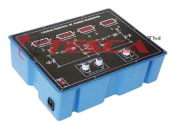
46561 Power Electronic Training Board has been designed specifically to study Power Transistor input and output Characteristics in common Emitter Configuration and Switching Characteristics of NPN Transistor. The board is absolutely self contained. Practical experience on this board carries great educative value for Science and Engineering Students.
