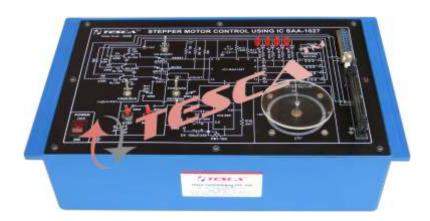
Stepper Motor Control trainer are based on IC SAA-1027 & designed to study the various functions of a stepper motor. It can be interfaced with microprocessor trainer and personl computer.
