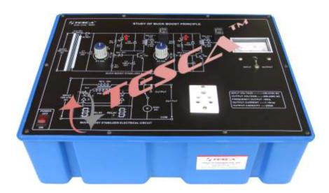
Study of buck boost principle has been designed with a view to provide practical/experimental knowledge of Automatic two step Buck Boost Principle with electronically controlled circuit. All the components and test points of the Principle are spread on the panel at appropriate places. A diagram is neatly drawn on the panel.
