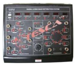
46609 Radial and Ring Main Distribution System is specially designed to illustrate the working phenomenon of Distribution System configured as Radial and Ring Main Distribution System. Distribution System is the part of electric power system which connects the high voltage transmission networks to the low voltage consumer service points. Distribution Systems should be designed in a way that Voltage variation at consumer terminals must be maintained with in ±5%.
