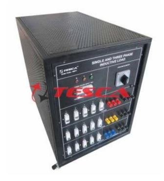
46611 Single and Three Phase Inductive Load is suitable for loading Single Phase and Three Phase supplies and generators. It consists of robust enclosure that contains three banks of switchable inductive loads. Two terminals for each phase are given which are externally accessible through an inbuilt star delta switch.
