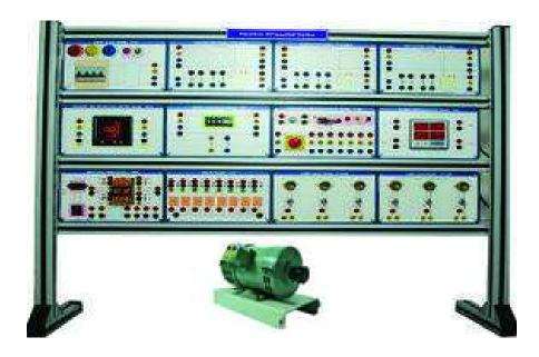
**46627A Industrial Installation Trainer** is a rouged training system for the Electrical laboratories mounted on Aluminum profile rack with sturdy table top flat panel. Each panel has ABS molded plastic sturdy enclosure with 4mm shrouded connectors showing circuit diagram & its connection tag numbers for easy understanding and connections. The product helps you to get fully acquainted with the basic concepts and functioning of an Industrial Installation Trainer.
