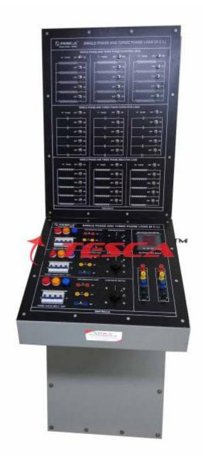
46650 Single and Three Phase Load is a high wattage network suitable for loading Single Phase and Three Phase supplies and generators. The load banks are used to verify the performance of power sources. However real loads are unpredictable and random in value hence standard loads are used to stimulate environment for testing power sources.
