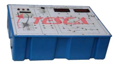
46710 Power Electronic Training Board has been designed specifically for the study of Three phase firing circuit for three phase ac voltage controller (without Neutral Configuration). Practical experience on this board carries great educative value for Science and Engineering Students.
