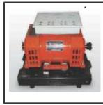
DC INTEGRATED (TRUNION MOUNTED) MOTOR Voltage : Varm= 180V Vfield = 180V Capacity -300W/2 Pole m/c, RPM - 1500, Shrouded Socket - 12 Rotor Construction: Standard commutator / brush arrangement with laminated stack, brought out on 2 terminals Stator construction : Separately excited field winding with laminated solid yoke 2 pole and series winding brought out on 4 terminals. Toque characteristic: Provision of load cells 6 Kg. 2 No. assembly to measure the torque.
