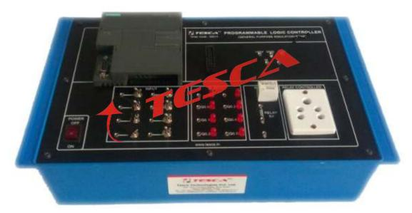
In today's the importance of PLC has rapidly increased with growing demand for training in this area. The standard packages for PLC are module experiment PCB, power supply, programming and operating software. Optional accessories includes digital and analog expansion modules.
