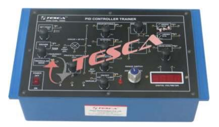
In control system there are different types of controller. Study of two-position mode as ON/OFF controller and continuous controller modes as PID controller is a very important part of control engineering. To have a basic idea and practical hands on controllers our PID Trainer has been designed to be used by student to investigate the fundamental principles of PID by applying different signals to it.
