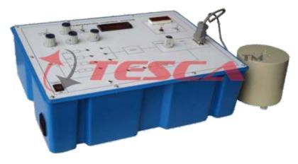
52033 Temperature control is an important application of control theory to industrial processes. This experiment has been designed to expose the students to such a practical control system, its various stages for control, and the tuning of a PID controller. The process consists of a small and fast responding oven which can be controlled in the temperature range from ambient to about 90°C.
