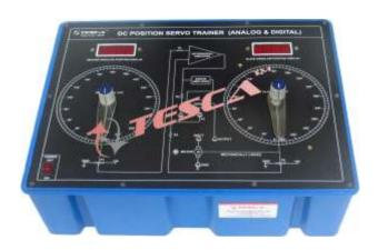
**Order Code** 52054 DC Position Servo Trainer (Analog & Digital) is designed specifically for the study of DC Servo Trainer and its use in Angular Position control. This Trainer covers the fundamental facts of DC Servo Trainer and its characteristics this trainer makes the student familiar with the DC Angular position control & DC Servo System. Four experiments can be performed by the trainer.
