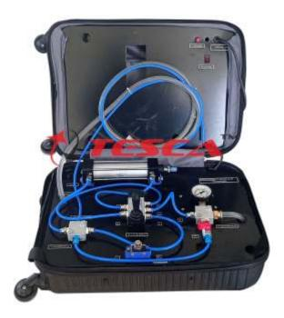
The Mini-hydraulic trainer is designed to study & understand various such basic components used while automation. The trainer consists of actuating devices, controlling devices, accessories, gauges, regulating devices and fitting & hoses. Basic purpose of the trainer is to give student an exposure to various hydraulic components & its principal of working and operation.
