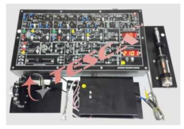
**52085** is a Sensor Trainer offer Complete training opportunity for most commonly used Sensor available for experimenting in the Laboratory. Due to the typical Strength obtain from a sensor is not enough to process the signal; this board provides signal conditioners with Digital panel meter for display.
