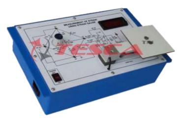
52089 provides study of Strain Gauge and their application for measurement of Strain, It helps to study bridge configuration of Strain Gauge and the signal conditioning circuits required to measure Strain. It uses cantilever beam arrangement to produce Strain on Strain Gauge.
