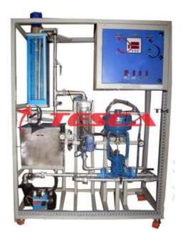
The Level Control Trainer is the system, which outlines the basics of Closed Loop Level Control and various aspects related to it.
