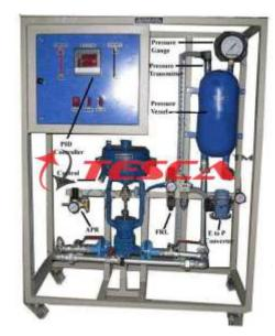
The Air Pressure Control Trainer is the system which outlines the basics of Closed Loop Air Pressure Control and various aspects related to it.
