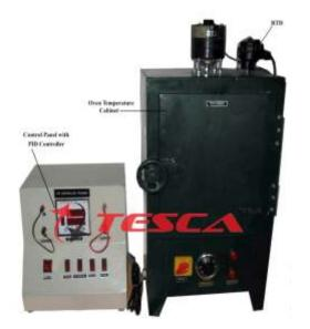
The Air Temperature Control Trainer is the system, which outlines the basics of Closed Loop Air Temperature Control and various aspects related to it.
