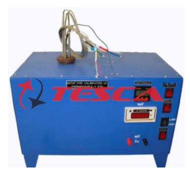
The Calibration of Thermocouple, RTD setup (52077-52280) gives an idea regarding calibration procedure for temperature transducers such as RTD, Thermocouple & Thermisters.
