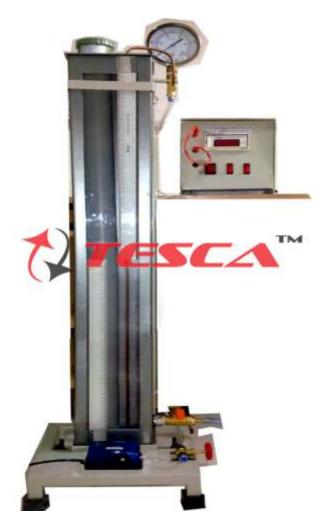
The Setup for Level Measurement using Ultrasonic Transducer (52311) gives an idea regarding Level Measurement based on Ultrasonic Principle.
