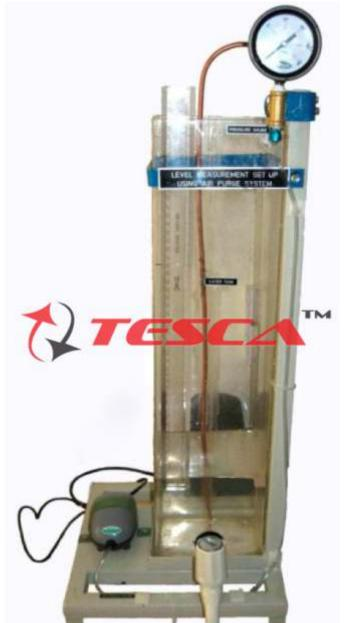
The Air Purge Bubbler System for Level Measurement Trainer (52317) is the system, which outlines the basics of level measurement using Air Purge method and other aspects related to it.
