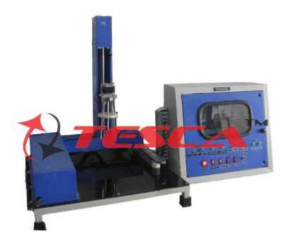
The Pick & place robotic application trainer (52319) gives provision to interface PLC with X-Y-Z Three axis displacement and a robotic arm.
