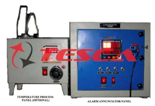
The Alarm Announciator Trainer (52361) gives idea regarding its use in industry for monitoring, alarm and control process plant parameters.
