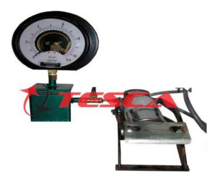
The set up gives an idea regarding the Operation of Bourdon Gauge Pressure sensor.
