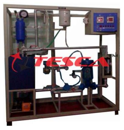
The Universal Process Control Trainer (52378) is highly flexible and modular system for studying of various feedback and cascade control loops in industrial processes. It has been designed to include these processes in a single structure. The system in fact includes transducers, PID + computerized control with SCADA Software.
