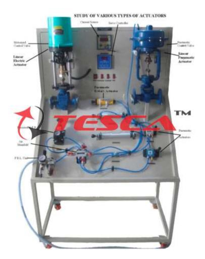
The Study of Various types of Actuators setup (52386) outlines the basic Principle of different Actuators used in Control System, & their applications.
