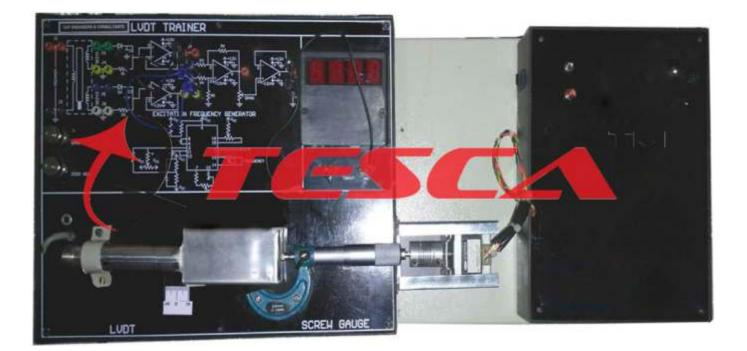
The **Displacement Measurement Motorized Bed Using LVDT** (52395) outlines the basics of Displacement measurement using LVDT.
