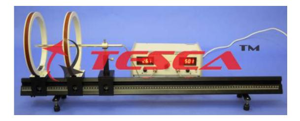
The experiment consists of two coils, Constant Current Power Supply and Gaussmeter. The Gaussmeter probe is mounted on a rail with a scale. It can move smoothly and precisely for measurement of magnetic field along the centre of the coils.
