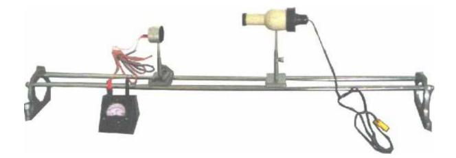
55701 Experimental Set Up has been designed specifically to study Selenium Photo Cell. The set up is absolutely self contained and requires no other apparatus.
