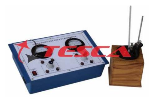
55702 Experimental Set Up has been designed specifically to determine the power factor of an A.C. circuit using Joule's Calorimeter. The set up is absolutely self contained and requires no other apparatus. Practical experience on this set up carries great educative value for Science and Engineering Students.
