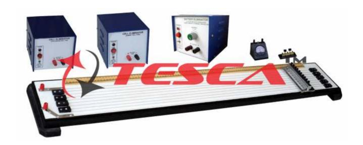
55712 Experimental Set Up R has been designed specifically for comparison of Electro Motive Forces (EMFs) of two primary cells by using a Potentiometer. The set up is absolutely self contained and requires no other apparatus. Practical experience on this set up carries great educative value for Science and Engineering Students.
