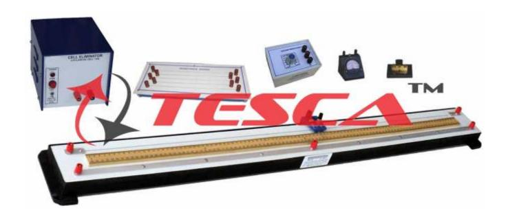
55723 Experimental Set Up has been designed specifically to verify laws of resistance inseries & parallel combination using a Meter Bridge. The set up is absolutely self contained and requires no other apparatus. Practical experience on this set up carries great educative value for Science and Engineering Students.
