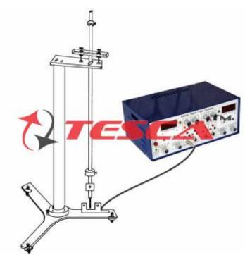
55734 Experimental Set Up has been designed specifically to study the viscous fluid (air) damping of a compound pendulum. It also aims at determining the damping co-efficient and Q of the oscillator. The set up is absolutely self contained and requires no other apparatus.
