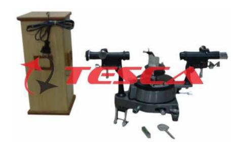
55750 Experimental Set Up has been designed specifically for the Measurement of Refractive Index of glass in the form of prism by Spectrometer. The set-up consists of Spectrometer, Mercury light source, Prism, Reading lens etc. The set up is complete in all respect and requires no other apparatus.
