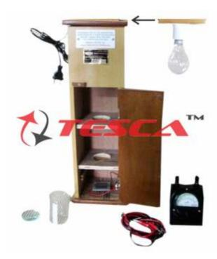
55757 Experimental Set Up has been designed specifically to determine the absorption coefficient of a liquid or solution with the help of photo voltaic cell. The set-up consists of photo voltaic cell, microammeter, glass vessel, light source etc.
