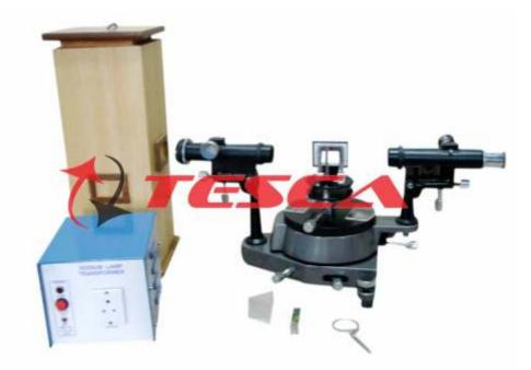
55760 Experimental Set Up has been designed specifically for the Measurement of Wavelength of sodium light by Diffraction Grating Method. The setup consists of Spectrometer, Diffraction Grating, Sodium light source, Prism, Reading lens etc.
