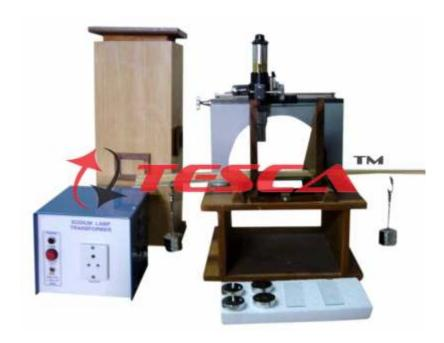
55762 Experimental Set Up has been designed specifically for determination of the Young's Modulus Y of Glass by Cornu's method. The set-up consists of Traveling Microscope, Sodium light source, Screw gauge, Vernier callipers, Glass plate, Wooden platform, Glass reflector & Weights with hangers etc.
