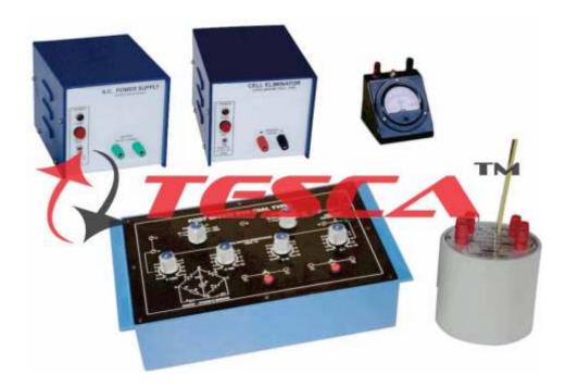
55780 Experimental Set-Up has been designed specifically to determine the temperature coefficient of resistance of conductors like copper and iron. The set up consists of P.O. Box, Galvanometer, Thermometer and Stirrer, Two conductors, Lenlanche cell, Oil bath container, etc.
