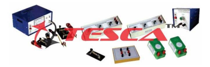
55788 Experimental Set-Up has been designed specifically to compare the capacities of two condensers by the method of MIXTURES using Electronic Coulombmeter, in place of conventional Ballistic Galvanometer. The set-up consists of Electronic Coulombmeter, two resistance boxes, Battery eliminator, one double pole double throw (D.P.D.T) switch.
