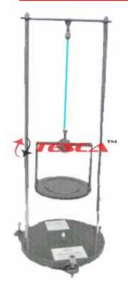
55793 Experimental Set-Up has been designed specifically to determine the moment of intertia (I) of a given body with the help of an Inertia Table.
