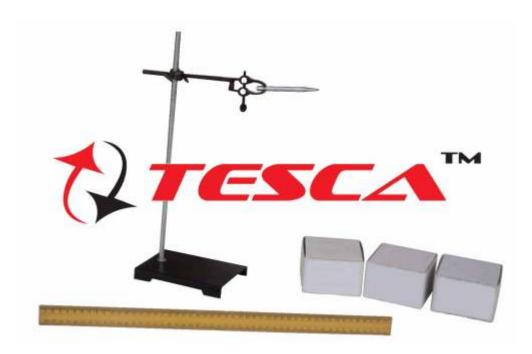
55799 Experimental Set-Up has been designed specifically to determine the refractive index of a liquid using a Concave Mirror.
